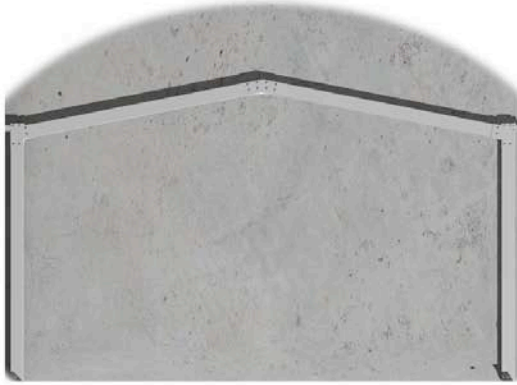
ASSEMBLE PORTAL FRAME ON THE GROUND
