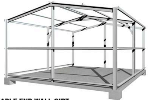
GABLE END WALL GIRTS IN PLACE
