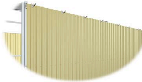
DISTRIBUTE HALF OF THE GUTTER BRACKETS EVENLY DOWN EACH SIDE WALL
